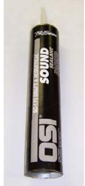
**Acoustic Sealant is a necessary component for stopping sound from leaking within wall systems. It is essential for achieving high STC value for total sound control. Leaving either a 1/4" or 3/8" bead at the drywall joints and installing acoustic sealant will increase the overall wall system performance by 12%. Acoustic Sealant is highly recommended to complete a vinyl sound barrier installation.**
