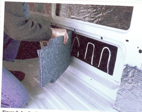
Figure 9. Application of Cascade Audio's Acoustical Cotton using heavy-duty construction adhesive (ICI Paints' Liquid Nails PN LN-903) was used to bond the Acoustical Cotton to the VMAX.
