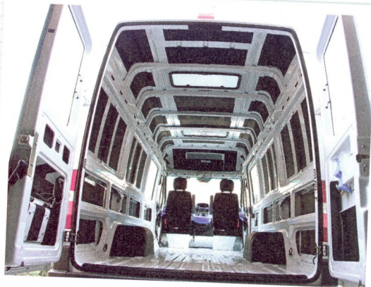
Figure 8. Cascade Audio's VMAX applied to cargo area walls.
